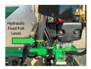
4. Hydraulic oil fill cap is located to the left of the dashboard. To fill the reservoir with new oil, use a small funnel to avoid spillage. Hydraulic oil capacity is 1.75 US gallons (15W 40 fully synthetic hydrostatic oil). Once filled, remove funnel and replace fill cap. Wipe all surfaces clean to remove residual oil.
