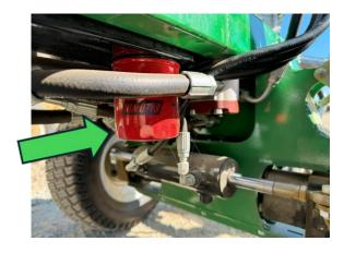
3. Replace the hydraulic oil filter (**Baldwin Part** #**BT8409 or Equivalent**). Filter can be found on the bottom of the reservoir tank.
