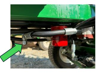
2. With oil drained and no oil continually flowing out of the fitting, replace the cap and tighten to ensure no further drainage.
