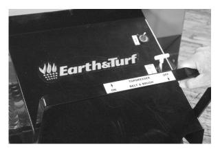
6 Ready to Spread - When you are ready to spread, you must engage the topdresser engagement lever rearward. To disengage the belt and brush, pull the lever forward. The topdresser will only spread when moving forward. The unit is designed this way so you cannot double-spread when backing into tight areas.
