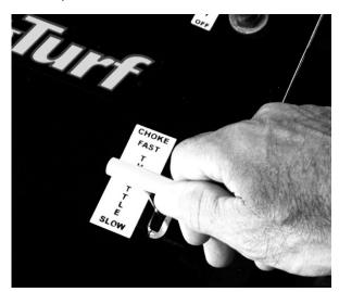
2 **Place the Throttle Lever** in the "choke" position and pull the starting rope, which is located just below the throttle control. When the engine starts, move the throttle lever back to the "fast" position.
