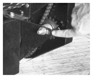
9 Brush Chain Tightness is adjusted by loosening the idler sprocket on the lower right side of the machine (viewed from behind the unit). Push the idler forward to tighten the chain, then re-tighten the idler bolt.
