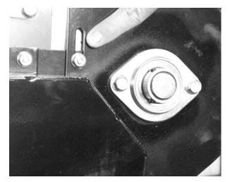
11 **Brush Adjustment** - The brush can be adjusted by loosening the nuts on the brush slide (one on each side of the unit). Push down on the brush assembly until the brush makes light contact with the conveyor belt,
