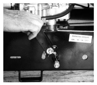
3 Release the Parking Brake by moving the lever backwards to the "off" position.
