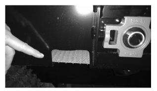
1 Clean the Belt & Roller Area after each heavy use with a pressure washer. Keep the engine running. Aim the wash stream on one side, then the other, moving it fore and aft until all material has been removed. To expose more of the roller, engage the machine, move it about 6 feet and repeat the washing procedure. Proper cleanout in this manner will help increase the service life of the conveyor belt.
