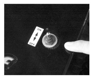
Engine On/Off Switch - After completing all necessary maintenance and making sure the fuel tank is full, start the engine by first positioning the toggle switch in the "on" position.
