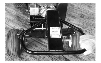
5 **Forward/Reverse** - To move the unit forward, push down on the steering handle. To steer the unit, simply move this handle from right to left, depending on the direction in which you wish to travel. To move in reverse, lift up on the handle and steer in the same manner.
