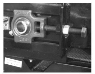
8 Conveyer Belt Adjustment is easily made by a single adjustment bolt on the left and right sides of the machine. First, loosen the jam nut and begin tightening the adjustment bolts. The belt should have some "play" in it. Each side should be adjusted the same, with the same distance between the bolt head and the front of the adjustment block. Having the adjustment equal on both sides is critical for proper belt tracking and acceptable service life of the belt.
