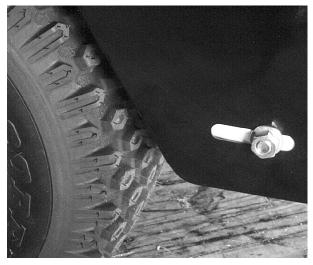
10 **Tightening the Conveyer Belt Drive Chain** is done by loosening the bolt that holds the chain idler (on the left side when viewed from behind the machine), then re-tightening the idler sprocket bolt.
