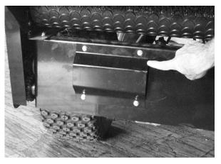
12 **Drive Clutch Service** - To access the overriding drive clutch, remove the four bolts from the back cover and remove the cover. This gives access to the clutch should repairs ever be necessary.
