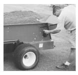
pulling the round knob to release the springloaded catch pin from its hole in the disc, then rotating the adjuster for proper endgate height. Release the pin and make sure it has been reset into one of the available adjustment holes.
